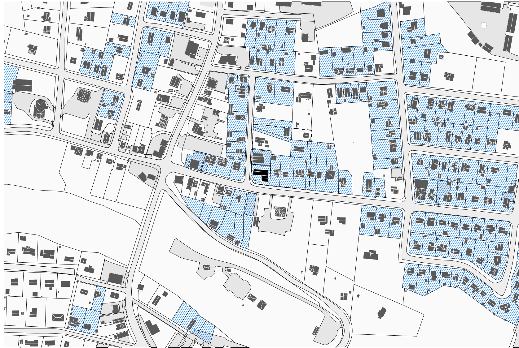
▨ NON-CONFORMING LOT AREA IN ZONING DISTRICT R1 EXISTING PARCEL REQUIRED PARCEL SIZE FOR USE GROUP (f) IN ZONING DISTRICT (R1)
